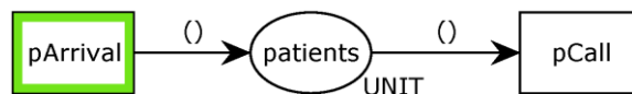
Figure 28. Petri net of the doctor’s waiting room system in its initial marking
